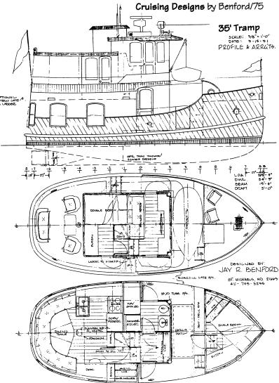
An alternative, for those looking for an even more "shippy" appearance, is the Tramp version, with a well deck about five feet long. The cargo hatch opens into an area below in which to stow diving gear, salvage treasures, or bicycles. The deck space can be used for lounging, carrying a personal watercraft, motorbike, or some extra fifty-five gallon drums of fuel or water.
